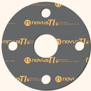
Novus TI is a graphite laminate product reinforced with an insertion of tanged 0.10mm thick 316 stainless steel. No adhesive is required to bond the graphite layers to the tanged insert resulting in a sturdy gasket material with excellent mechanical strength.
