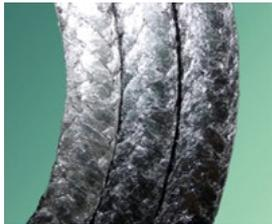
Novus Unipac 2 combines graphite yarn inserted with multi Inconel wires reinforcement to create a flexible braided graphite spool packing with increased extrusion resistance and higher pressure capability. This Packing does not have any fiber carrier in all its twisted yarn. Novus Unipac 2 unique construction increase extrusion resistance, thus eliminating the need for separate anti-extrusion rings. The increased extrusion resistance also increases the maximum pressure rating without end rings.
