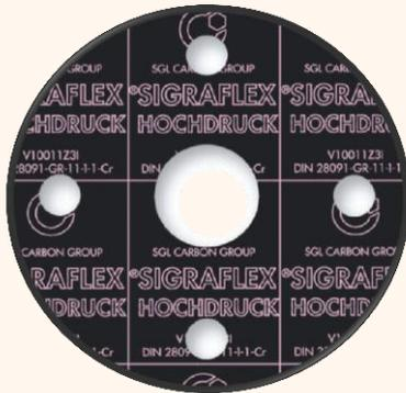
*Sigraflex Hochdruck® is a multi-layer sheet material comprising 0.5mm thick layers of high quality graphite foil and 0.5mm thick stainless steel foil. Depending on the sheet thickness required, several layers of graphite and stainless steel foil are joined together in a special process without the use of an adhesive. The result is a sealing material with outstanding mechanical properties.*
