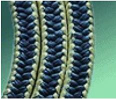
Novus Unipac 5 is a high-quality braided packing made of PTFE yarns fiber incorporated with graphite and reinforced corner yarns of Aramid fiber. It can prevent gaps from extrusions in the presence of high pressure and temperature. It has good sliding velocity and thermal conductivity. It enables to seal high pressure piston pumps during long running periods.
