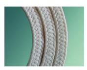
Made from reinforced acrylic fibre with over 60% concentrated PTFE dispersion with added break-in lubricant, lightly tensioned construction offers flexibility and compression for good sealing.
