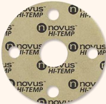
Novus Hi-Temp consists of Phlogopite mica paper impregnated with a high quality silicone binder. Mica is a aluminosilicate of mineral origin, which has a lamellar and non-fibrous structure representing an excellent alternative to asbestos at high temperatures. This material gives Novus Hi-Temp its thermal characteristics - weight loss at 800°C(1472°F) less than 5% - and its chemical resistance to solvents, acids, bases and mineral oils.
