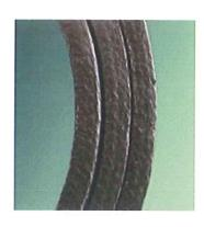
Made from reinforced acrylic fibre, each strand of yarn is sealed off with a special grade of fine graphite flakes. In addition, a final coating of graphite is given to final product prior to its being squared.
